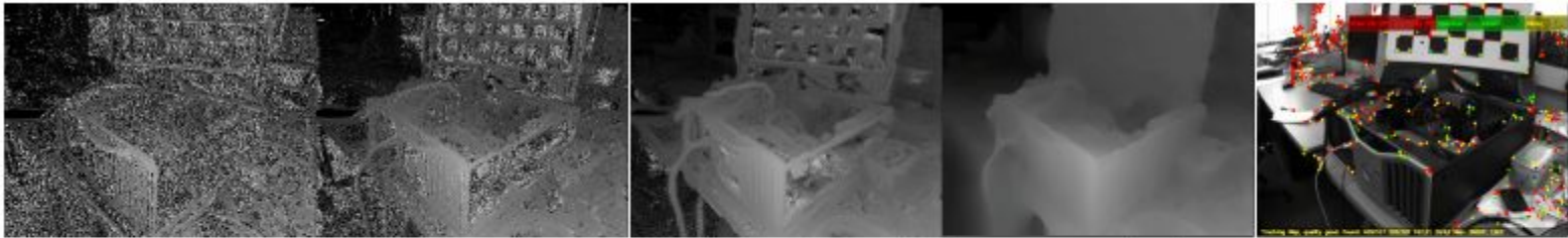
Figure 3. Incremental cost volume construction; we show the current inverse depth map extracted as the current minimum cost for each pixel row d_{\mathbf{u}}^{min} = \arg \min_d \mathbf{C}(\mathbf{u}, d) as 2, 10 and 30 overlapping images are used in the data term (left). Also shown is the regularised solution that we solve to provide each keyframe inverse depth map (4th from left). In comparison to the nearly 300 \times 10^3 points estimated in our keyframe, we show the \approx 1000 point features used in the same frame for localisation in PTAM ([6]). Estimating camera pose from such a fully dense model enables tracking robustness during rapid camera motion.
